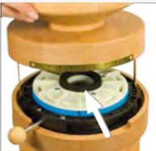
Figure 9 Make sure the foam rubber gasket is properly seated (arrow). Return the funnel to its previous position and secure it with the brass screws.
