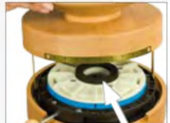
Figure 4 Make sure the foam rubber gasket is properly seated (arrow). Return the funnel to its previous position and secure it with the brass screws.
