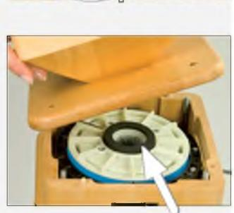
Now return the funnel to its previous position and secure it with the brass screws
